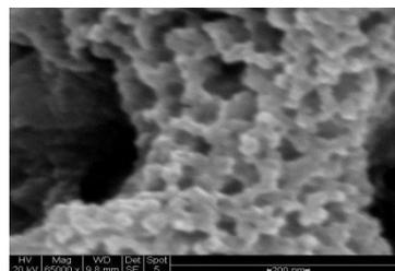
Figure 3: SEM micrograph of activated carbon of coir fibre
