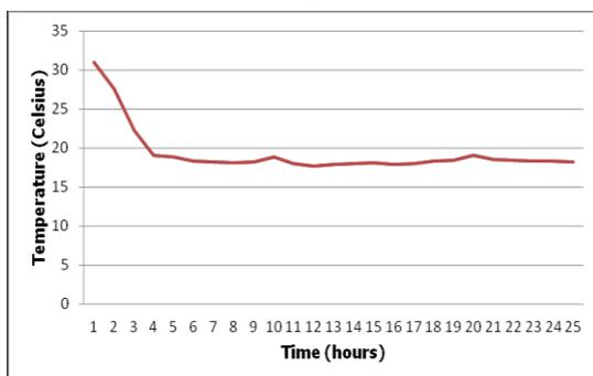
**Figure 2. Variation of the temperature inside the cooling chamber over 24 hrs of period.**
