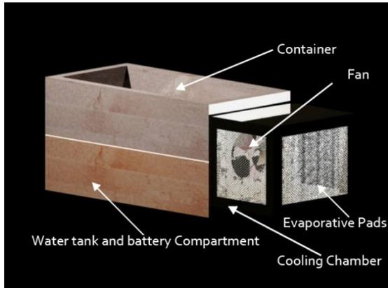
**Figure 1. View of evaporative cooler**
