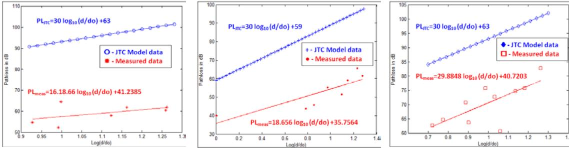
Figure 2: Pathloss variation according to the measured and JTC data for 3<sup>rd</sup>, 2<sup>nd</sup> and 1<sup>st</sup> floors
