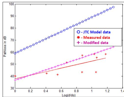
Figure 3: Comparison of measured and modified data of EDISIL access point
