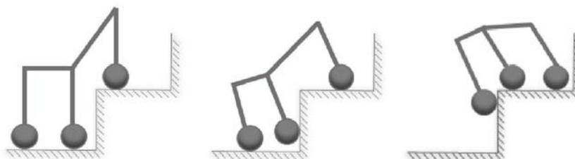
Fig. 1: The concept of the flexible structure hugging the step as it moves forward making its ascent.
