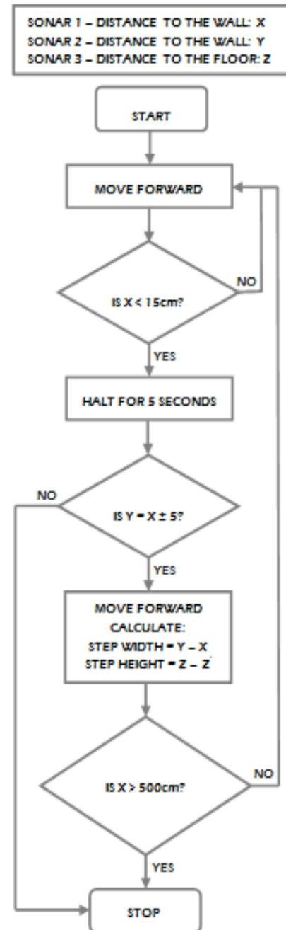
SONAR 1 AND 2 FOLLOW THE SAME VERTICAL ALIGNMENT BUT SONAR 1 IS POSITIONED NEAR BOTTOM RIM OF WHEELS WHERE AS SONAR 2 IS POSITIONED AT THE HEAD OF THE ROBOT.
