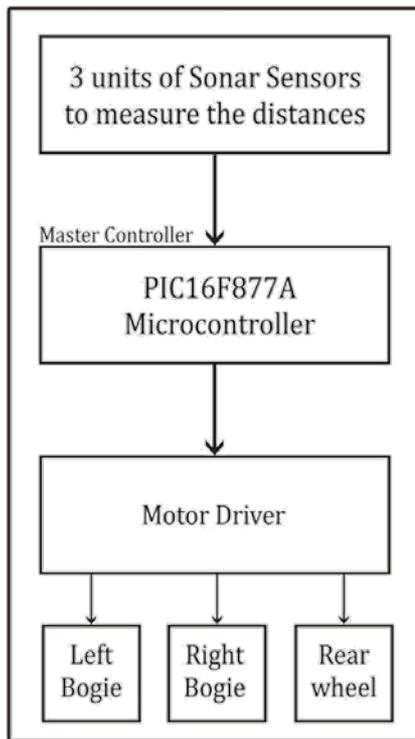
Fig. 2: Schematic of the control system
