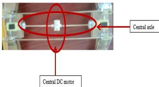
Figure 3.3-Power transmission
