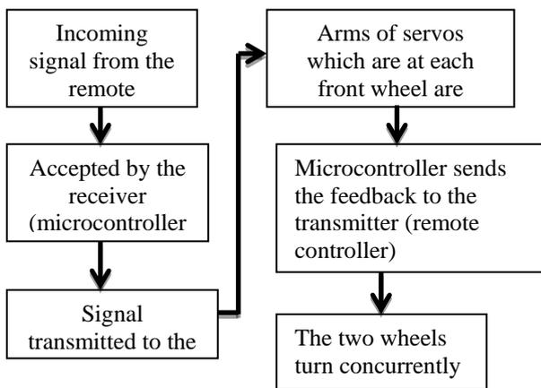
Figure 2.2: The simple flow diagram below indicates how the steering is done.
