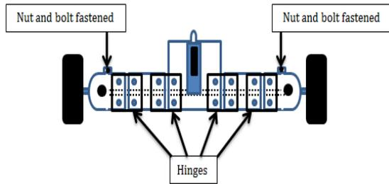
For the **rear wheel** drive, nut and bolt were used to restrict steer enabling motion.
