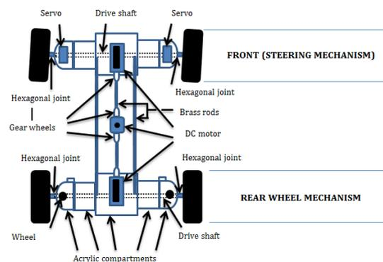
Figure 1: Mechanical sketch (Block diagram) (not drawn to scale)
