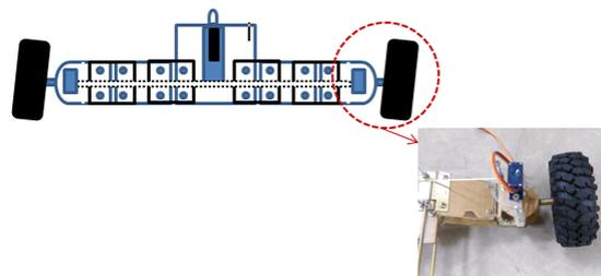
Figure 3.2.a-Steering mechanism
