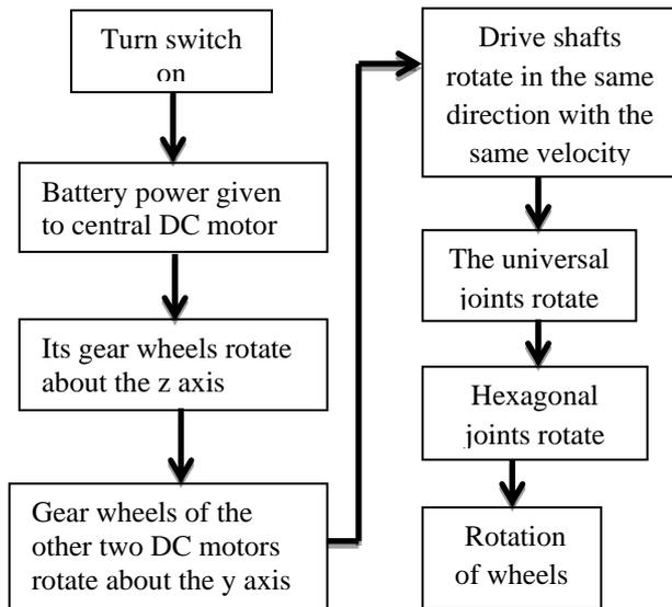
Figure 2.1: Overall sequence of events to drive the wheels of the UGV.
