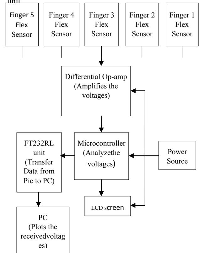
Figure 03: Main components of the glove
