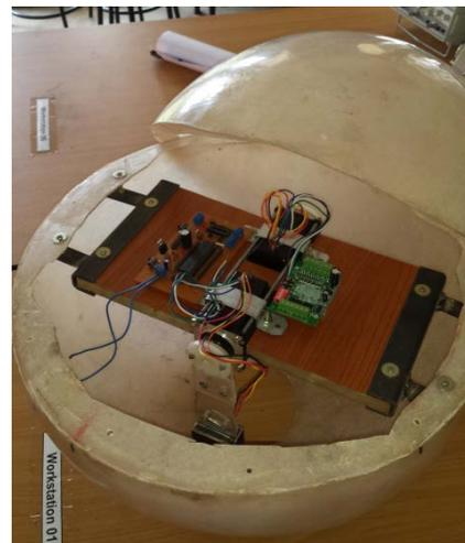
Figure 1 Spherical mobile robot
