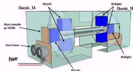
Figure 3: Components of the individual modules
