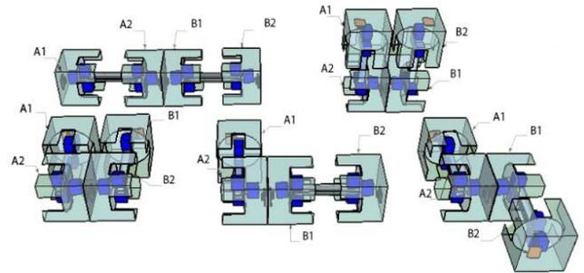
**Figure 5: Different transformations available with 2 modules**
