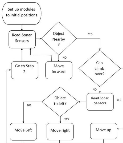
**Figure 4 : Program Flowchart Showing Overview of Robot Operations**
