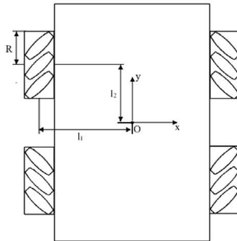
Figure 4: Basic schematic of the robot chassis
