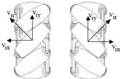
Figure 3: The velocity components of the mecanum wheel ( $i = 1,2,3,4$  depending on the wheel)
