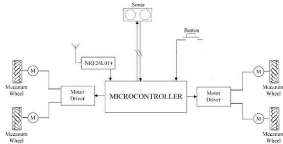
Figure 8: Block diagram of the robot
