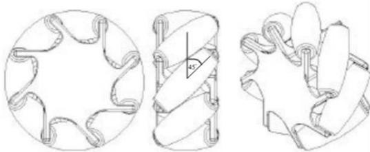
Figure 2: Drawing of the mecanum wheel
