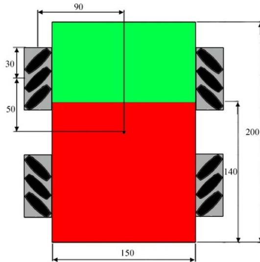
Figure 7: Top view of the chassis (Note that the sketch is not to scale)
