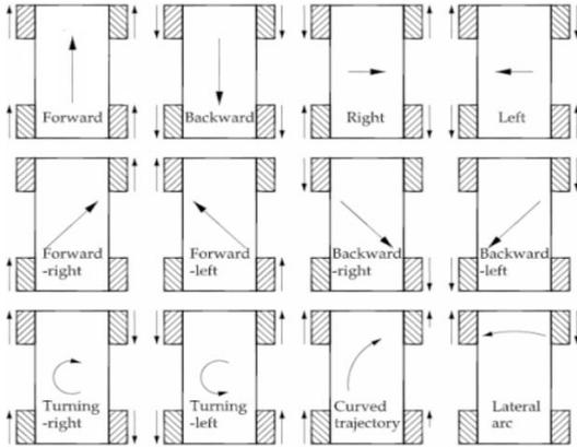
Figure 5: Diagram depicting the different motor controls to achieve different directions[4]
