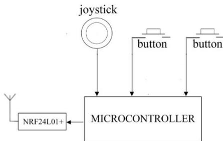
Figure 9: Block diagram of the remote control
