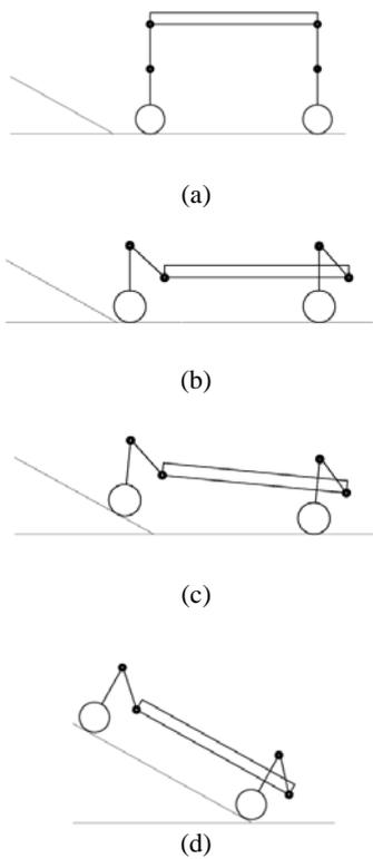
Figure 6: Incline plane traveling mechanism.
