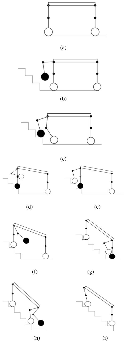
**Figure 5: Step climbing mechanism**
