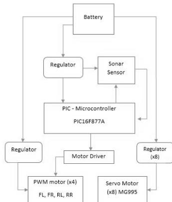
Figure 8: Block diagram
