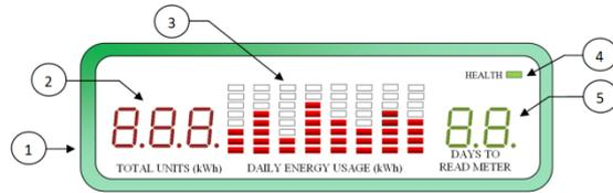
Figure 5: Front panel of Energy Monitor
