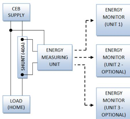
**Figure 2: Smart electrical energy monitoring system**
