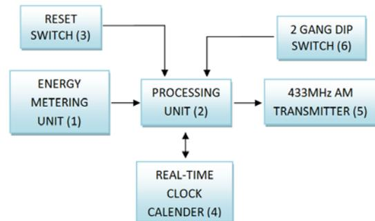
**Figure 3: Energy measuring unit**
