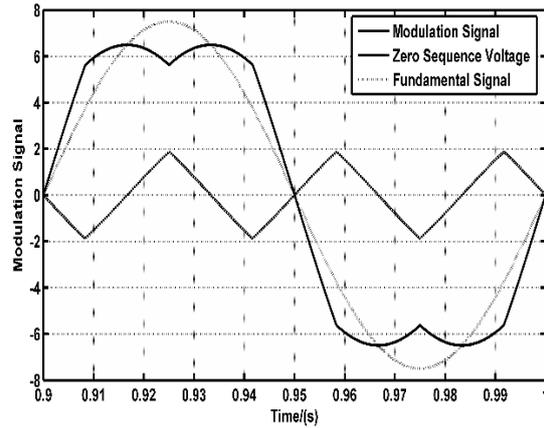
**Figure 4: Symmetric PWM generation signals**
