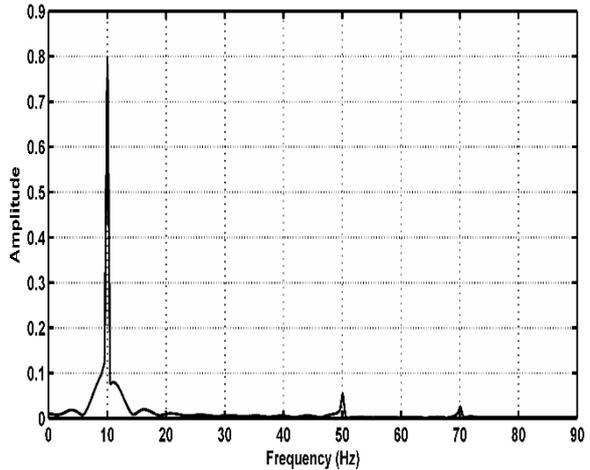
**Figure 8: Single-Sided Amplitude Spectrum of Distorted Phase A Current**
