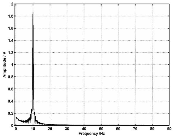
**Figure 9: Single-Sided Amplitude Spectrum of Compensated Phase A Current**
