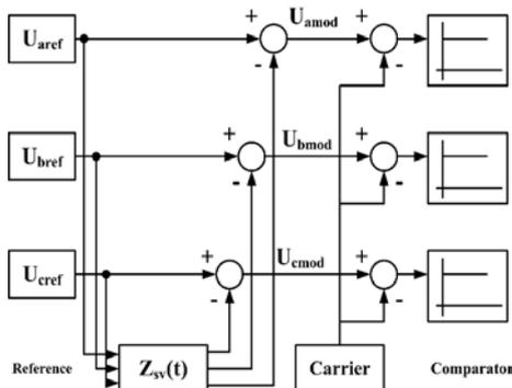
**Figure 3: Symmetric PWM generation signals**
