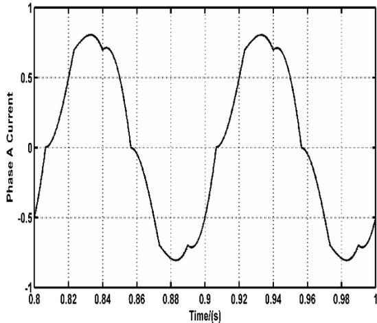
**Figure 6: Distorted Phase A Current Waveform**
