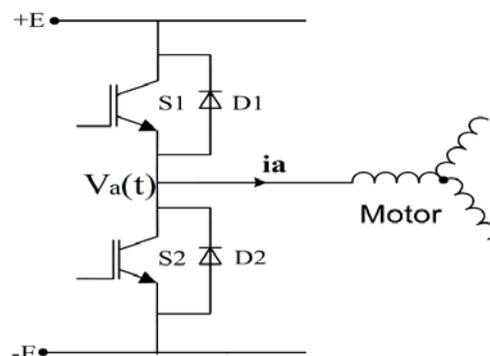
**Figure 1: One Leg of the Three Phase PWM Inverter**
