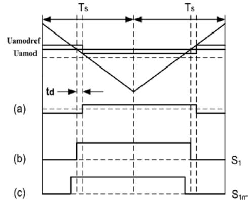
**Figure 5: Phase Lag Elimination Method**
