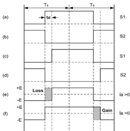
Figure 2: Distorted PWM gate signals
