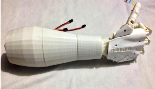
**Figure 2: Complete 3D printed robotic hand**
