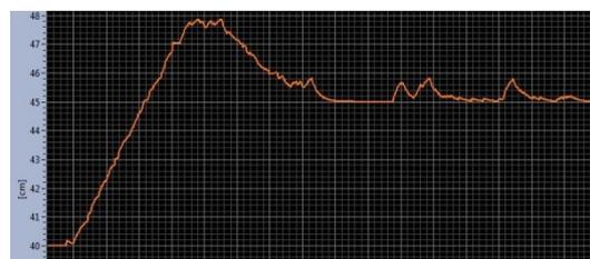
Figure 9: Performance response using Z-N method
