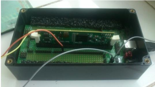
Figure 3: TI Delfino F28355 Experimental kit
