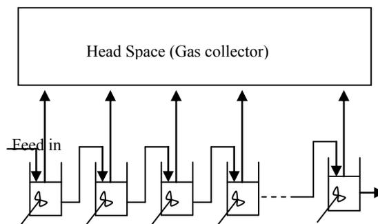
**Figure 2: Schematic model of CSTR in series reactor arrangement (n=10)**
