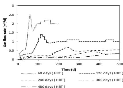
**Figure 3: Variation of biogas production rate in PFR under varying feed rates**
