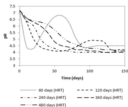
**Figure 5: pH variation of the plug flow reactor at front**
