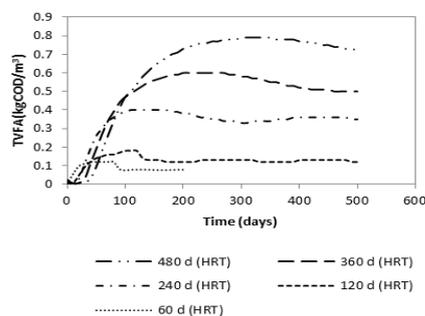
**Figure 4: Total VFA variation at the front of the reactor**
