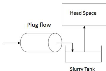
**Figure 1: Schematic model of advective diffusive reactor with slurry collection tank and gas collection tank**
