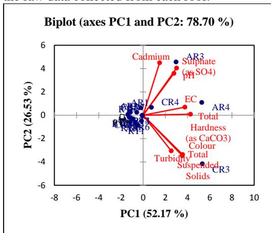
**Figure 7: Biplot from the Principle Component Analysis (PCA) of all the data collected from all three roofs. (RT-Tile Roof, AR-Asbestos Roof, CR-Corrugated Steel Roof, EC- Electrical Conductivity)**
