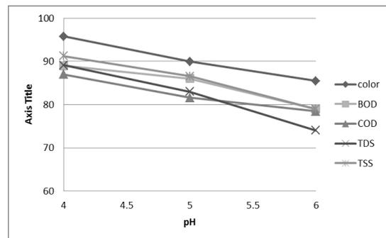
**Figure 5: Initial pH against the % removal of BOD, COD, TDS, TSS, and Color using 1.2ml and 90g of coagulant-adsorbent**
