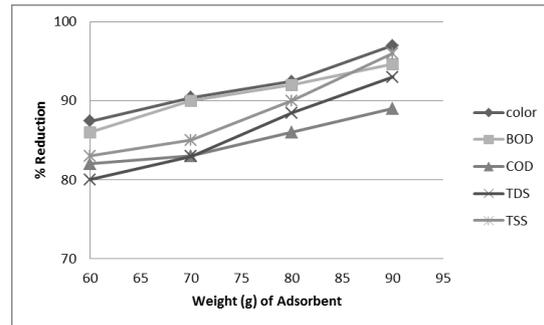
**Figure 4: Concentration of adsorbent as weight (g) against the % removal of BOD, COD, TDS, TSS, and Color at constant pH and Coagulant concentration**
