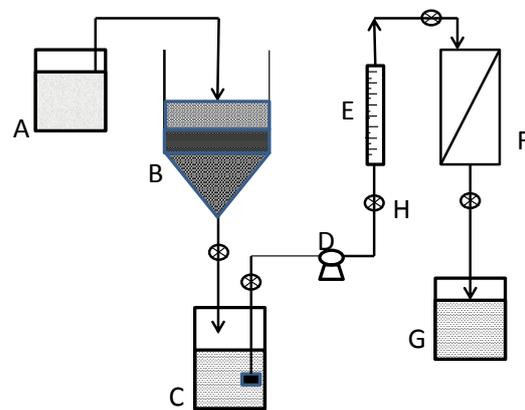
**Figure 1: Schematic diagram of physical treatment system developed in this study : (A) Solution obtained after jar test chemical treatment ; (B) dual media gravity filter ; (C) Water collection tank after gravity filter ; (D) Centrifugal pump of 0.5hp ; (E) Rota meter to adjust the exit flow rate ; (F) Micro filter ; (G) Product collection tank ; (H) Valves**
