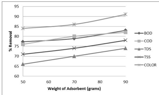
**Figure 2: Weight (g) of 355  $\mu\text{m}$  Adsorbent against the % removal of BOD, COD, TDS, TSS and color**
