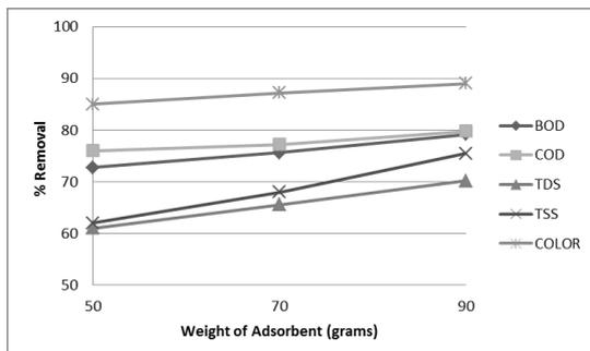
**Figure 3: Weight (g) of 500  $\mu\text{m}$  Adsorbent against the % removal of BOD, COD, TDS, TSS and color**
