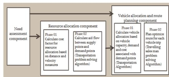
Figure 1: Design of the optimization tool
