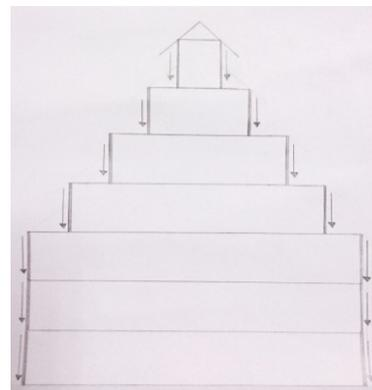
**Figure 6: Load is transferred from seventh floor to the first floor through columns (Load path)**
