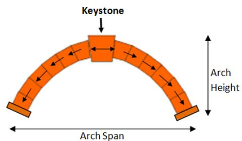
**Figure 5 :Show how the load is distributed from the keystone**
