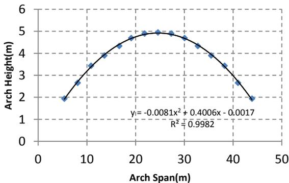
(c) Pilimathalawa truss-arch bridge : Parabolic shape
