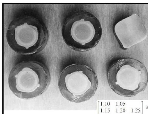
**Figure 1: Changes in martensite layer with the quenching time [3]**
