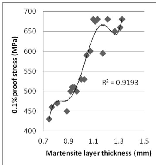
Figure 2: 0.1% proof stress vs. martensite layer thickness
