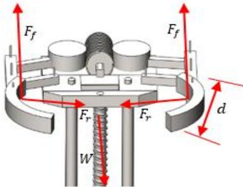
Figure 3: Force diagram of one platform
