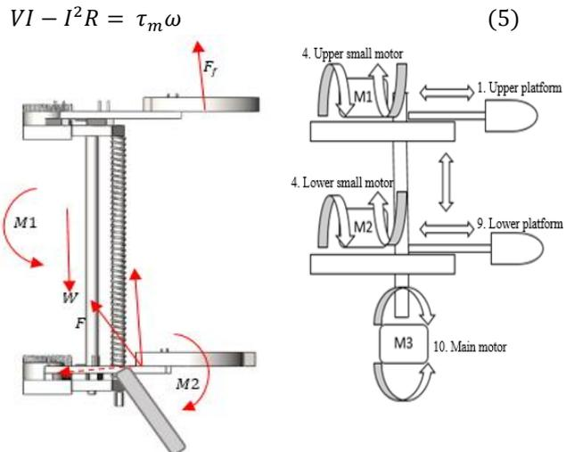
The minimum required torque of main motor is calculated by equation 5. In this case, power is used to rotate motors. The total consumed power ( $\tau_m \omega$ ) is equal to total input power ( $VI$ ) minus power losses due to coil resistance ( $I^2R$ ).
