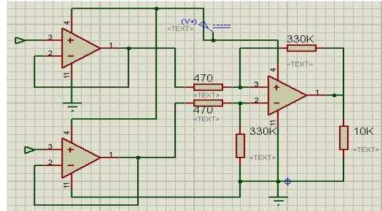
Figure 4: Load sensor and instrumentation amplifier diagram
