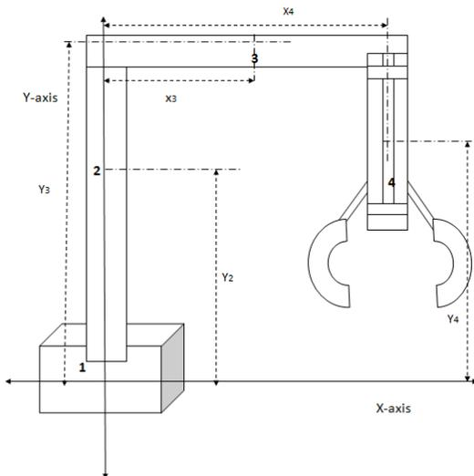
Figure6: Indicating dimensions that are needed for center of gravity calculations.
