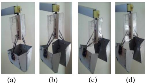
Figure 4: Figure (a) The completely closed position of the gripper. Figures (b) and (c) shows slightly opened positions of the gripper
