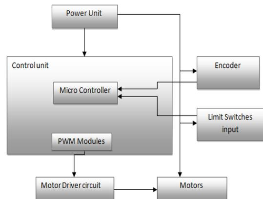
Figure 5: System architecture of the proposed gripper and pick and place mechanism.
