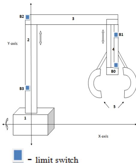
Figure 1: Design and Degrees of freedom. First degree of freedom is shown by the component 2 which will move along vertical axis and other
