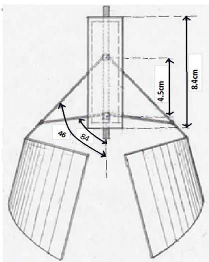
Figure 3.b: The dimensions of the fully open gripper.
