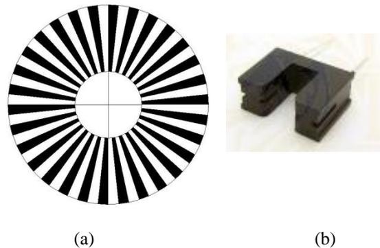
Figure 2: (a) encoder, (b) U-shaped IR sensor
