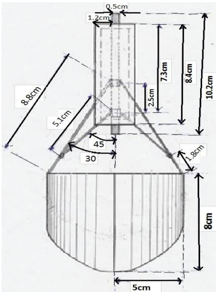
Figure 3.a: The dimensions of the gripper at the fully closed position.
