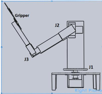
Figure 5: Mechanical Robot Arm Unit 2D View
