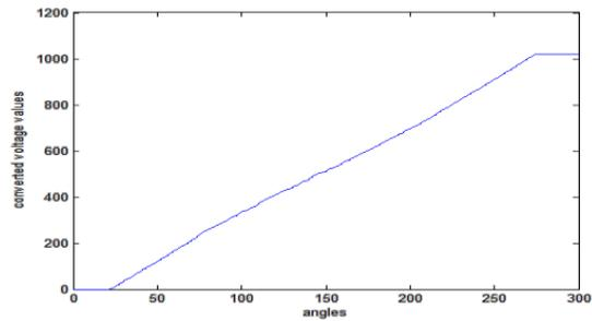
**Figure 3: The plot of variable voltage bits varying with angle**
