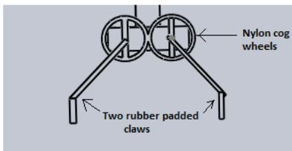
Figure 6: Mechanical Robot Arm Unit
