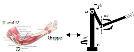
**Figure 2: Motion Capturing Wearable Structure side by side comparison with Human Arm**
