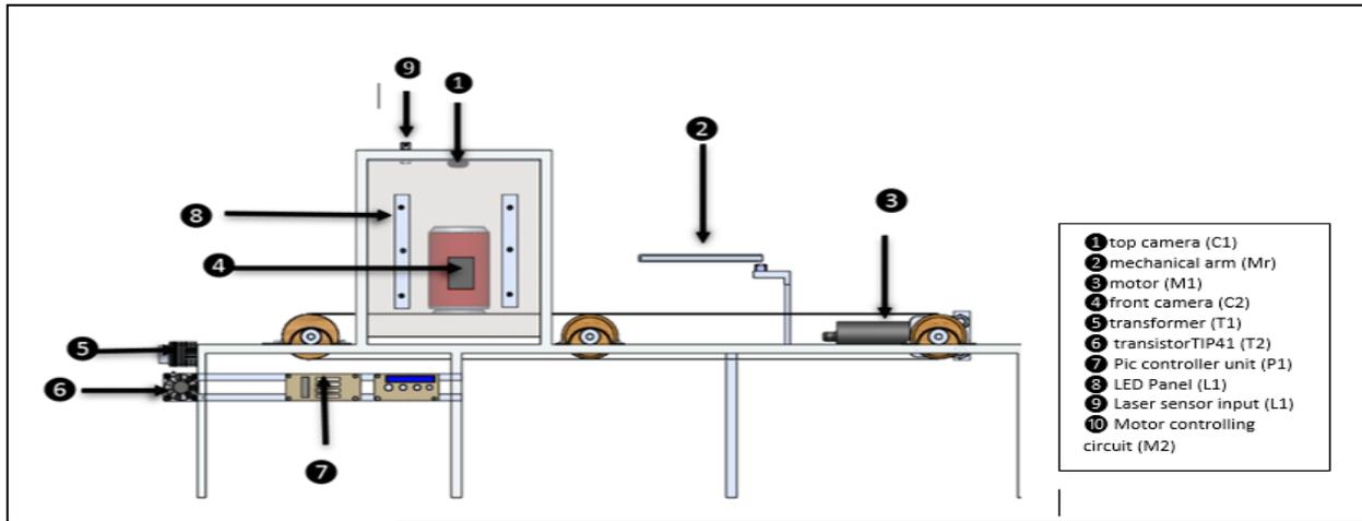
Figure 01: System Architecture
