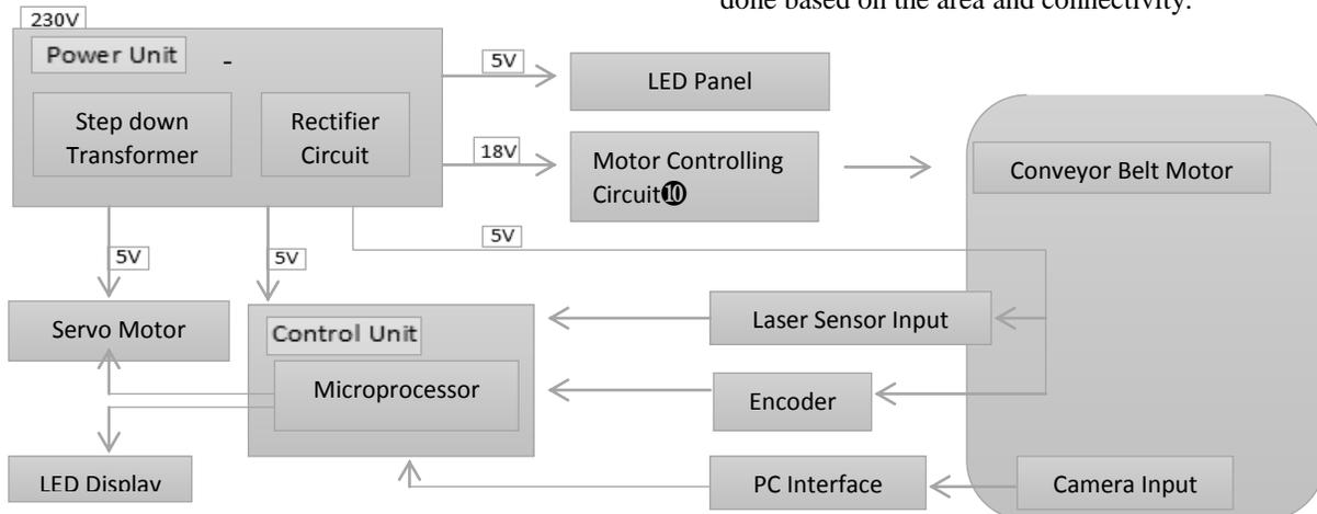
Figure 02: process flow diagram
