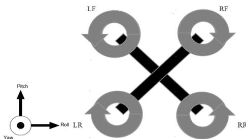
**Figure 1: Motor rotation directions of the Quadcopter; Motors: left front (LF), right front (RF), left rear (LR), right rear (RR).**
