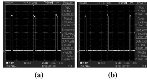
Figure 5: Change of Pulse Stream applied when configuring the ESC, (a) Maximum Speed, (b) Minimum Speed
