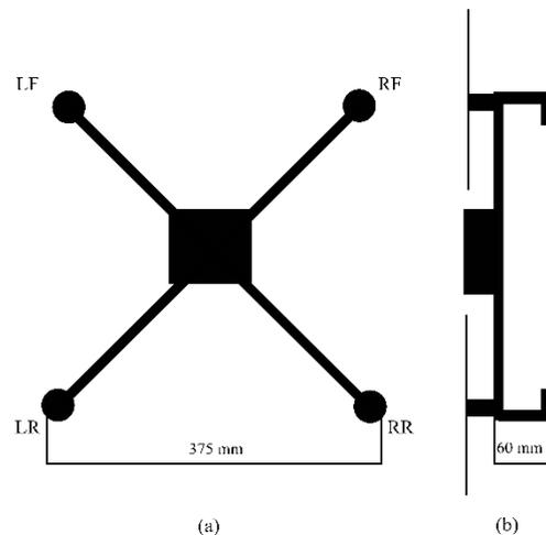
**Figure 4: The rendered image of the Structure with dimensions. (a) Top View showing all four motors, (b) Right Side View, showing the motors in right side, RF and RR.**
