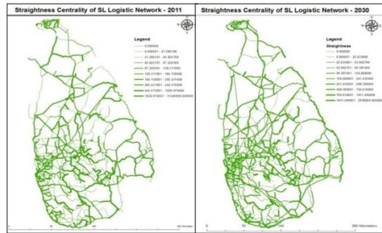
Figure 3: Straightness Centrality of Existing and Proposed Networks
