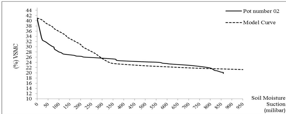
Figure 2: Soil moisture characteristic curve developed from lysimeter data and SPAW model
