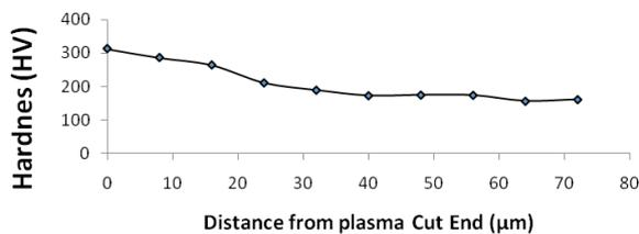
Figure 1.1 HARDNESS PROFILE FOR N1
