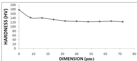
Figure 2.1 HARDNESS PROFILE FOR N2
