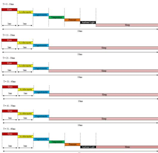
Figure 2: Data transmission sequence
