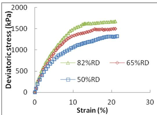
Figure 5: Deviatoric stress vs. axial strain plots for various BS+1%F mixes at different relative densities (400 kPa confining pressure)
