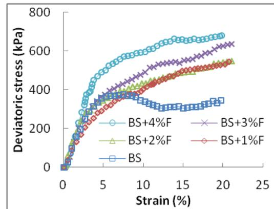
**Figure 3: Deviatoric stress vs. axial strain plots for various BS+F mixes at 50% relative density (100 kPa confining pressure)**
