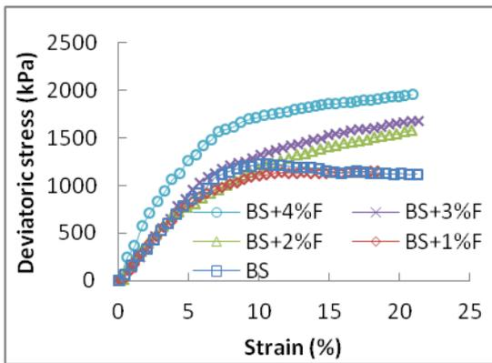
Figure 4: Deviatoric stress vs. axial strain plots for various BS+F mixes at 50% relative density (300 kPa confining pressure)
