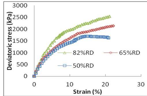
Figure 6: Deviatoric stress vs. axial strain plots for various BS+4%F mixes at different relative densities (400 kPa confining pressure)
