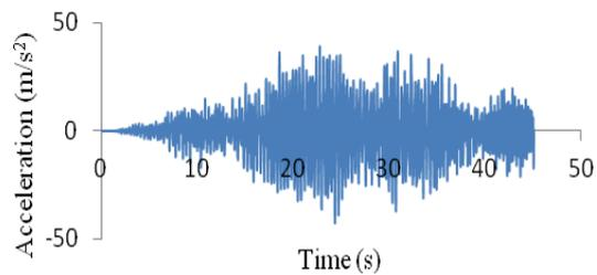
**Figure 5- Output acceleration-time history at top free surface.**
