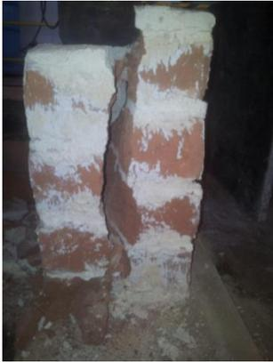
Figure 9: wall panel fractured due to compression loading
