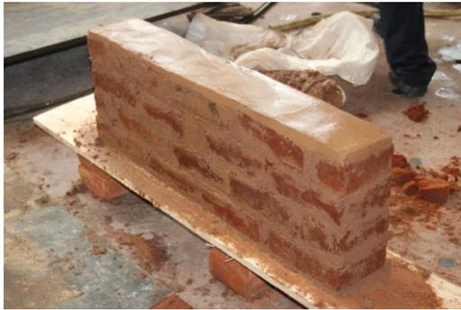
**Figure: 2** wall panel built using the ancient mixture
