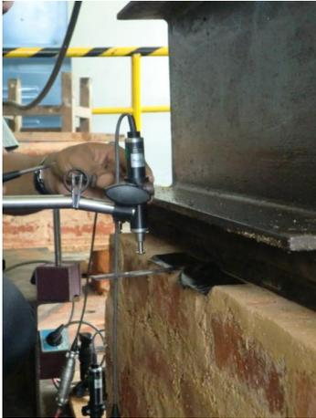
**Figure: 5 arrangements of displacement gauges for compression test**
