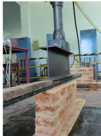
**Figure 4:** Testing arrangement for compression loading
