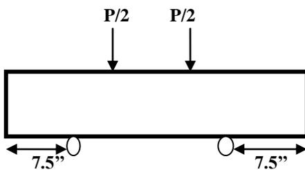
**Figure 6: Top view of the flexural testing arrangement.**
