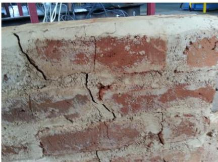
Figure 10: Tension cracks formed due flexural deformation
