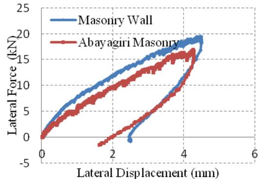
Figure: 11 Graph of loading and unloading of both walls
