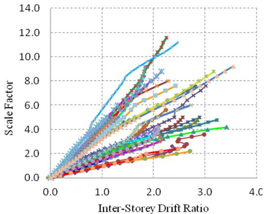
**Figure 3: Incremental dynamic analysis curves for 30 earthquakes**
