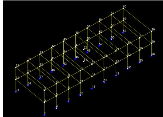
Figure 2: Numerical model developed in OPENSEES
