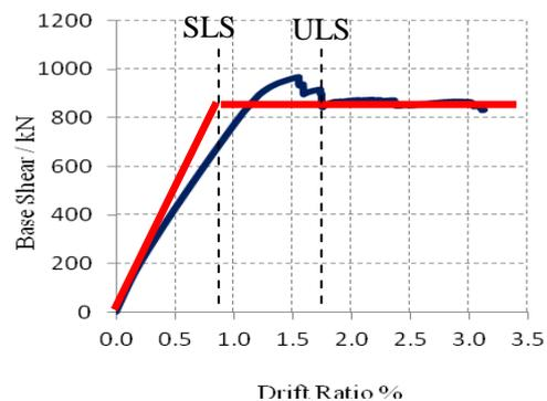
**Figure 5: Pushover curve and equivalent bi-linear curve**
