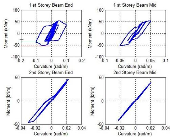
**Figure 4: Moment-curvature diagrams**
