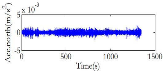
**Figure 5(a): N-S component of acceleration time history at top storey in building 2**
