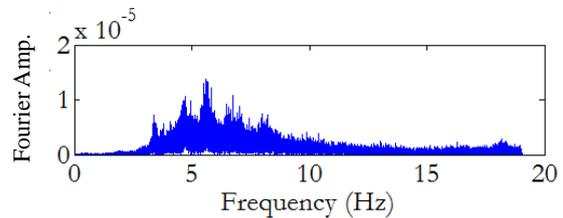
Figure 3(b): Fourier spectrum of N-S component of acceleration- building 1
