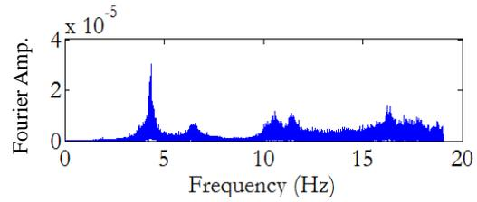
**Figure 6(a): E-W component of frequency time history at top storey in building 2 (1200 s)**
