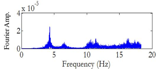
**Figure 6(b): E-W component of frequency time history at top storey in building 2 (300 s)**
