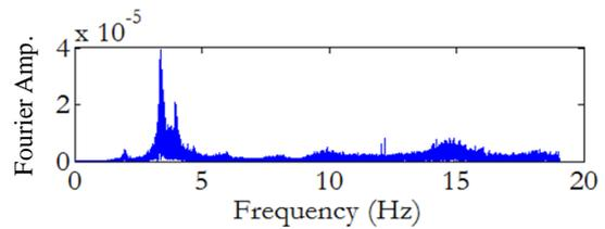
Figure 2(b): Fourier spectrum of E-W component of acceleration- building 1
