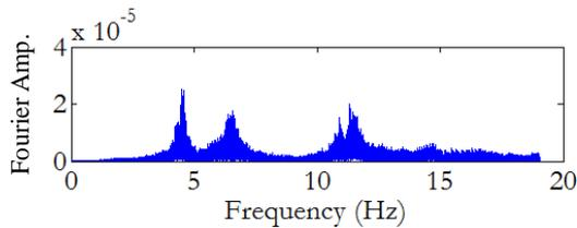
**Figure 5(b): N-S component of frequency time history at top storey in building 2**
