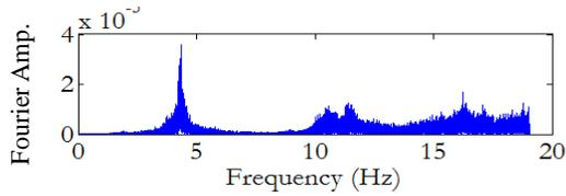
**Figure 4(b): Fourier spectrum of E-W component of acceleration- building 2**
