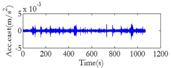
Figure 2(a): E-W component of acceleration time history at top storey in building 1
