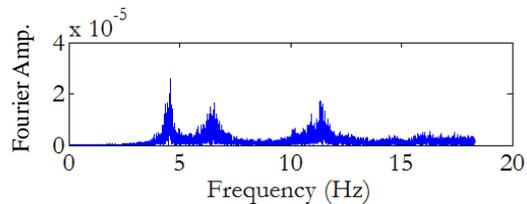
**Figure 7(b): N-S component of frequency time history at top storey in building 2 (300 s)**
