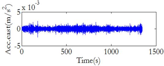
**Figure 4(a): E-W component of acceleration time history at top storey in building 2**
