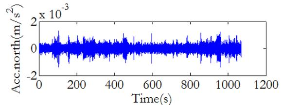
Figure 3(a): N-S component of acceleration time history at top storey in building 1
