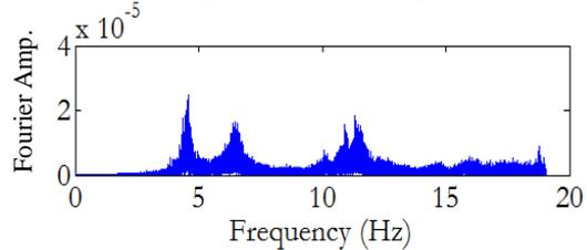
**Figure 7(a): N-S component of frequency time history at top storey in building 2 (1200 s)**
