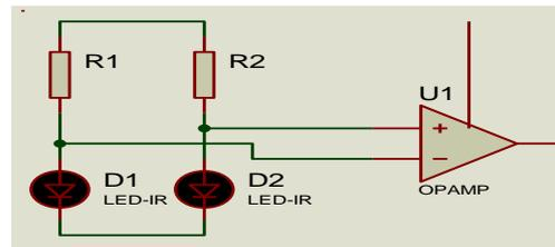
**Figure 3: Sensor interface amp circuit**
