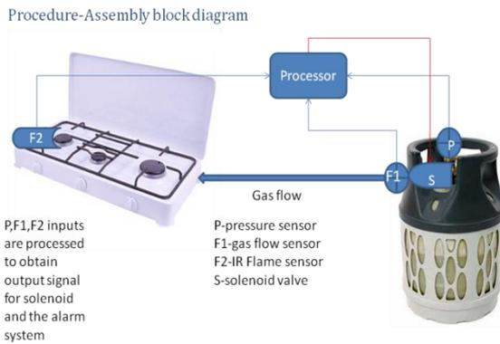
**Figure 1: Assembly Diagram**
