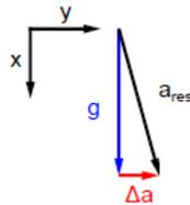
Figure 3: Small change in acceleration orthogonal to the gravity
