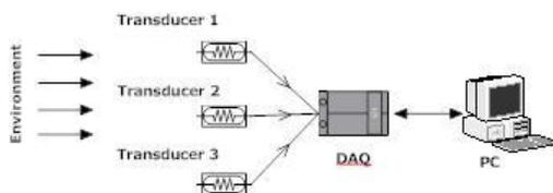
**Figure 1: Typical Data Acquisition Process**
