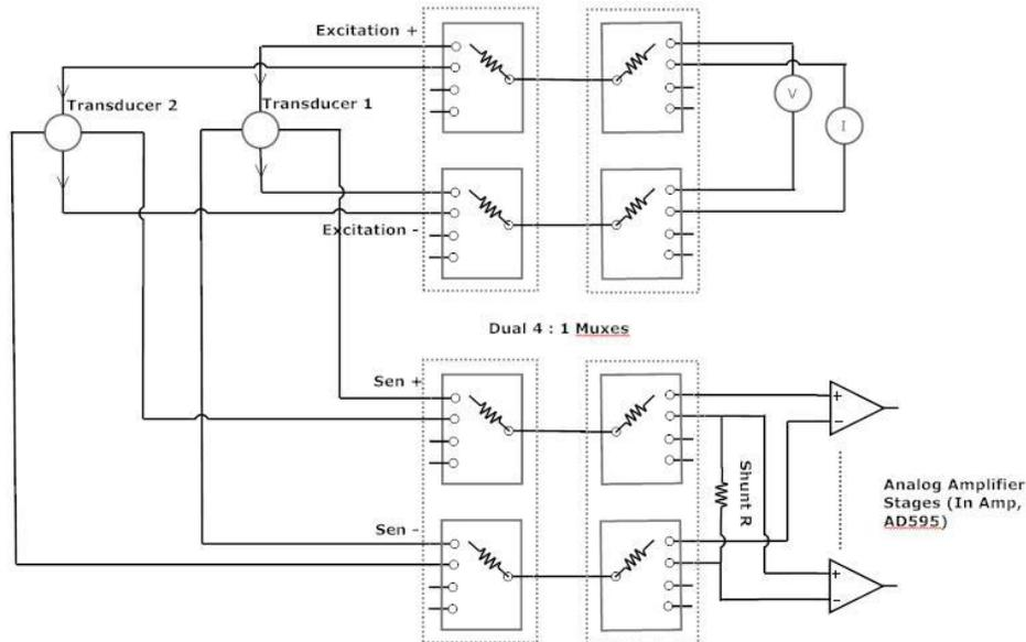
Figure 2: Universal Interface (4 Channel) based on Analog Multiplexer Network
