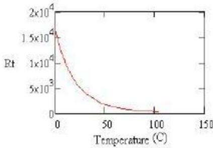
**Figure 3: Thermistor Response Curve**
