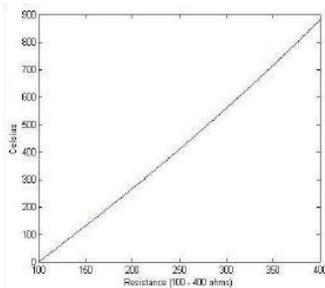
**Figure 4: Linearization of RTD Data**
