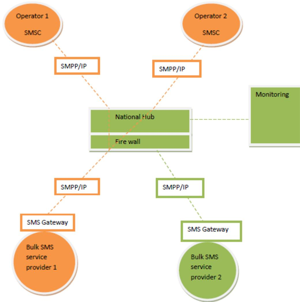
**Figure 2: The suggested architecture of Hub.**
