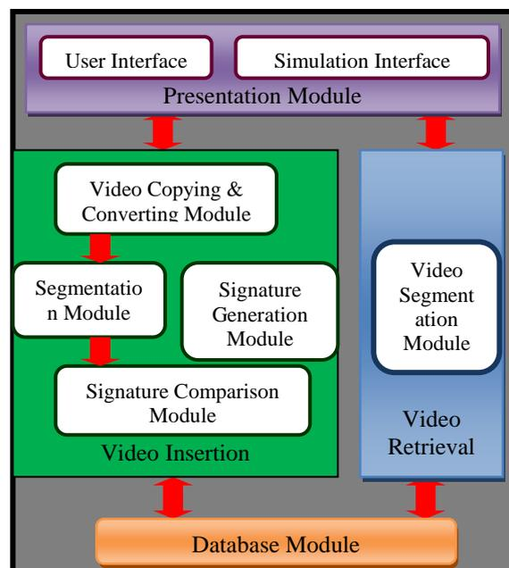
**Figure 1: Modular architecture of ATUWA video redundancy manager software**
