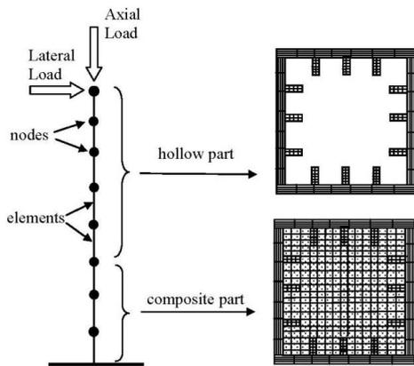
Figure 2: Finite element model of specimen N1
