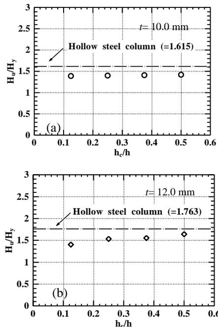
Figure 7: Variation of strength index with  $h/h_c$  ratio; (a)  $t=10.0$  mm; (b)  $t=12.0$  mm
