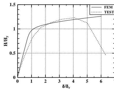
Figure 3: Comparison of test and analytical load-displacement curve for specimen N1
