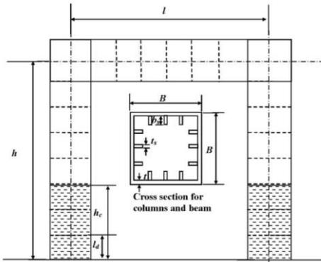
Figure 4: Concrete-filled steel rigid frame model
