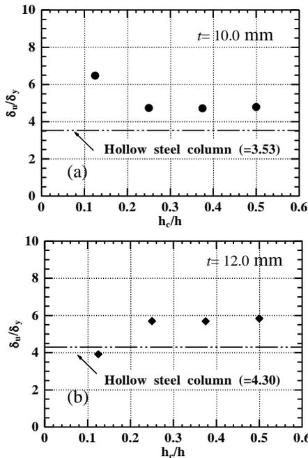
Figure 6: Variation of ductility index with  $h/h_c$  ratio ; (a)  $t=10.0$  mm; (b)  $t=12.0$  mm
