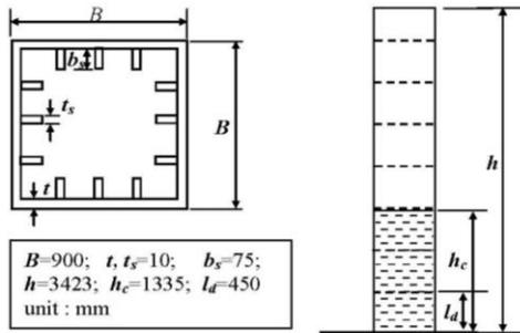
Figure 1: Geometry of test specimen N1 (Amano et al. 1998)
