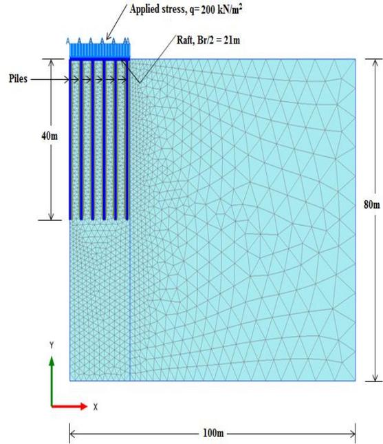
**Figure 1: Finite element mesh of piled raft foundation.**
