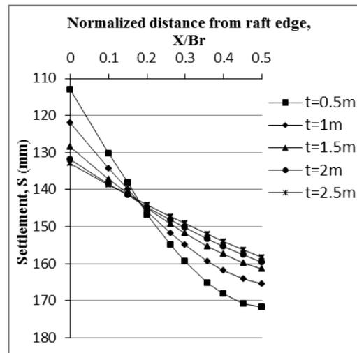
**Figure 2: Effect of raft thickness.**
