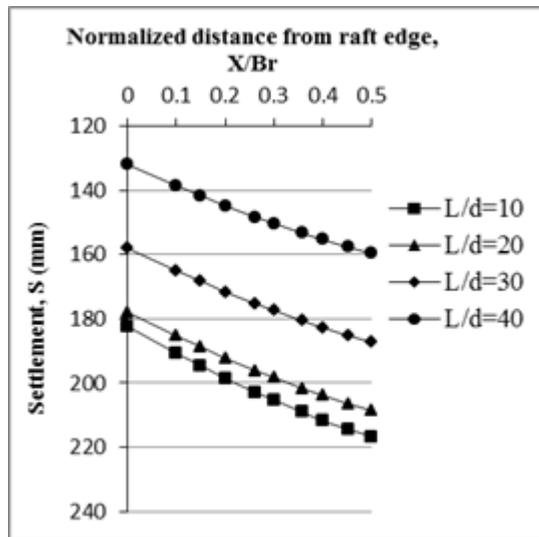
Figure 3: Effect of pile length
