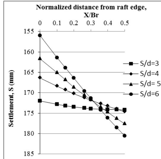
Figure 4: Effect of pile spacing
