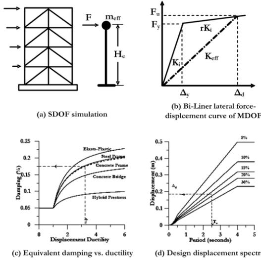
**Figure 1: Fundamentals of Direct Displacement-Based Design (Priestley, 2007).**
