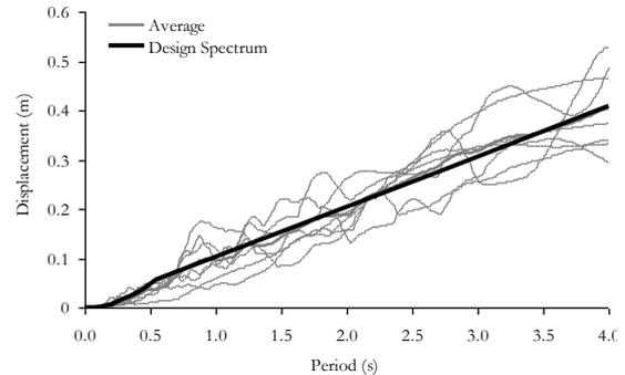
Figure 4: Displacement spectra from the scaled natural accelerogram at 5% damping
