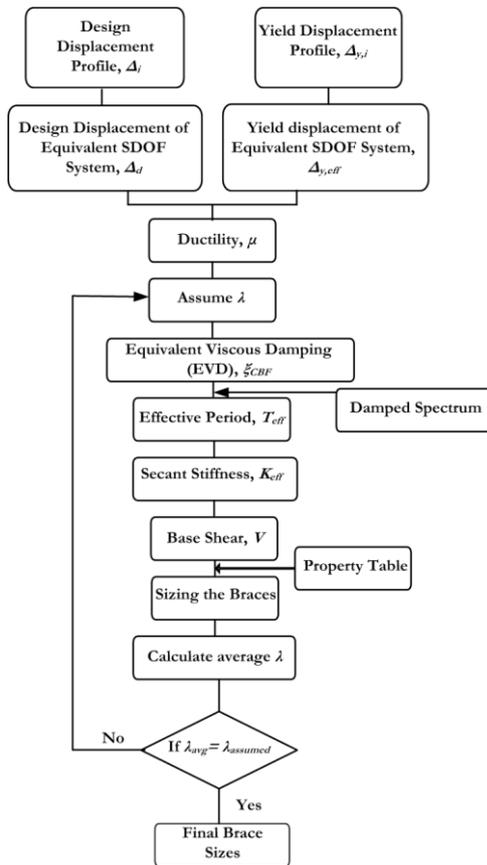
Figure 3: (a) Flow chart on DDBD procedure of CBF structures
