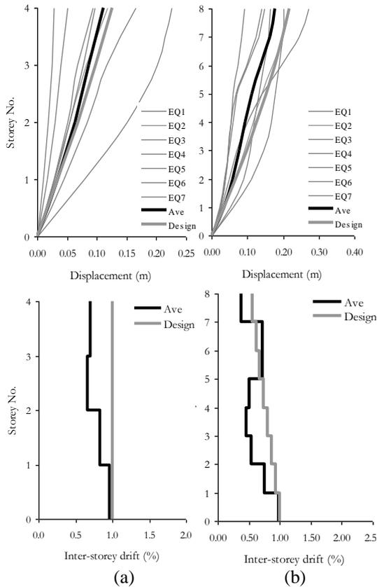
**Figure 5: Average peak displacement and drift ratio profiles of (a) 4 storey (b) 8 storey CBFs**
