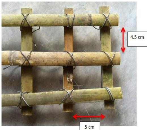
**Figure 2: Arrangement of the bamboo reinforcement layer**
