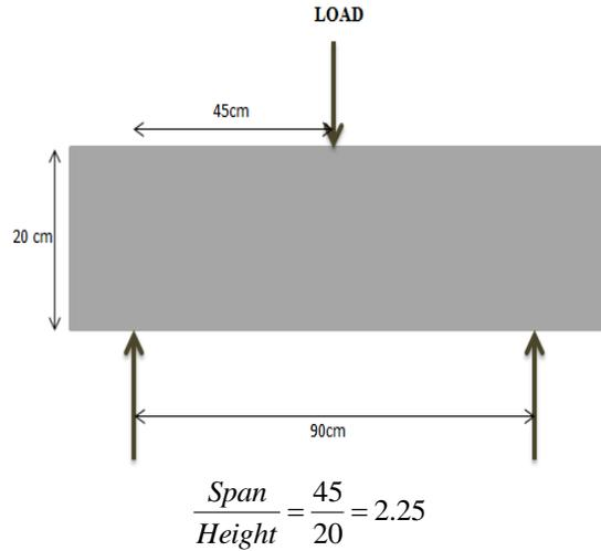
**Figure 3: Testing arrangement**
