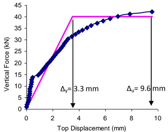
**Figure 4: Vertical force-deformation curve obtained from the experiment**
