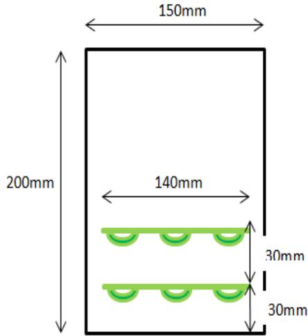
**Figure 1: Geometric characteristics of the bamboo reinforcing beam.**
