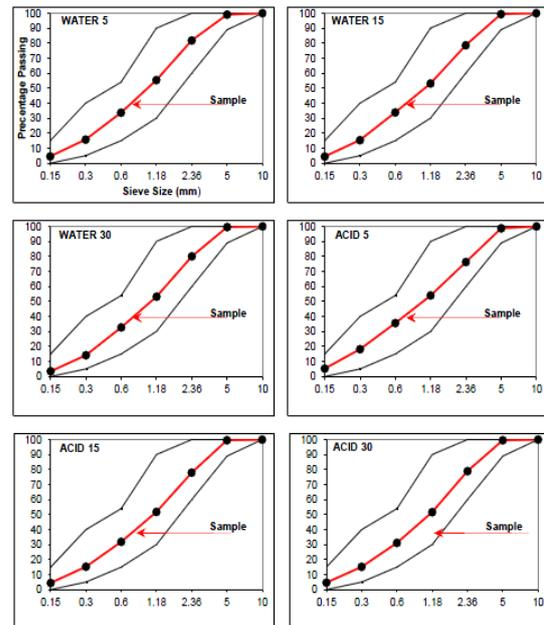
Figure 1: Particle size distribution curves of six categories of sand
