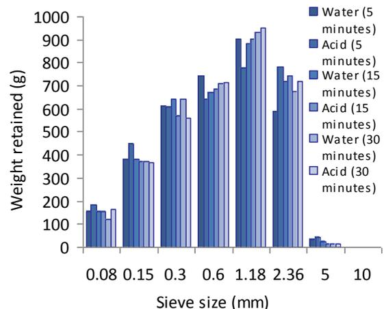
Figure 2: Weight retained in each sieve of each category of sand
