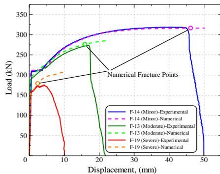
**Figure. 7: Comparison of load - elongation curves of proposed analytical model**
