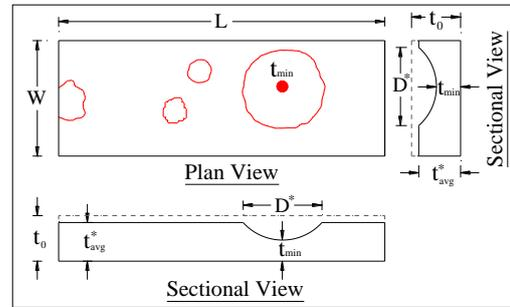
**Figure 5: Analytical model with CCM parameters**
