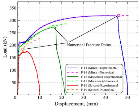
**Figure 3: Comparison of experimental and analytical load-displacement curves**
