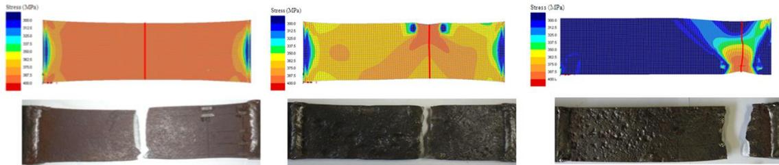
(a) F-14 [Minor corrosion] (b) F-13 [Moderate corrosion] (c) F-19 [Severe corrosion]
