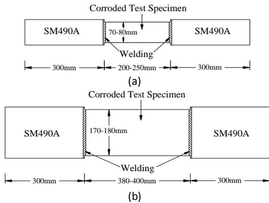
Figure 1: Dimensions of (a) flange and (b) web test specimens
