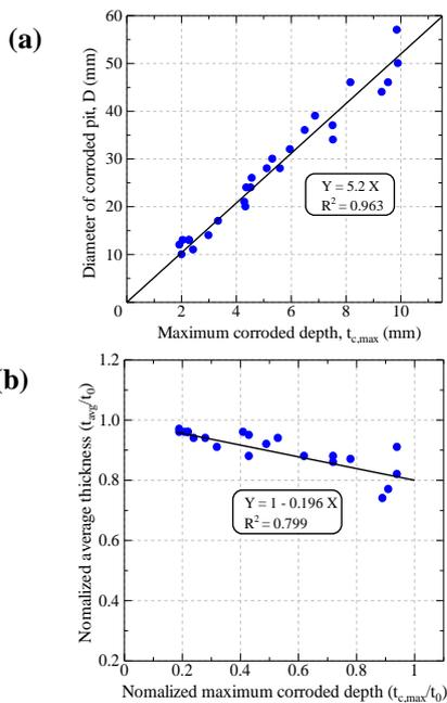
**Figure 4: Relationship of (a)  $D$  vs.  $t_{c,max}$  and (b) normalized  $t_{avg}$  vs.  $t_{c,max}$**
