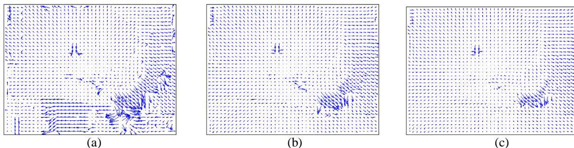
**Figure 4: A capture of motion estimated for 'Table tennis' sequence with (b)  $\lambda_E = 50$   $\lambda_R = 7$  and (c)  $\lambda_E = 150$   $\lambda_R = 11$  using the RDE optimisation, compared with (a) JM reference encoder output at similar RD performance (bit rate 600.44 kbps & PSNR 34.42 dB) at QP 30.**
