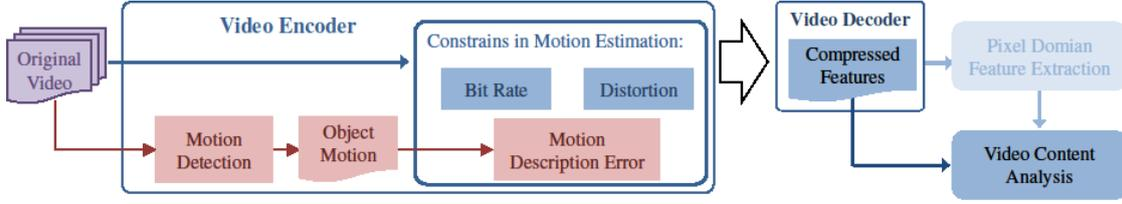
**Figure 1: Overview of the proposed encoder implementation with Rate-Distortion-Motion Description Error (RDE) optimisation**
