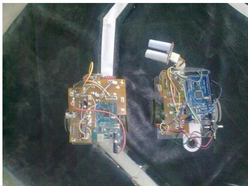
**Figure 3: Leader and Follower Robot in operation on Symmetric track**
