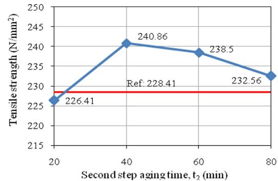
**Figure 5: Tensile strength Vs Second step aging time,  $t_2$**
