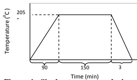
**Figure 1: Single step age hardening treatment applied in industry**
