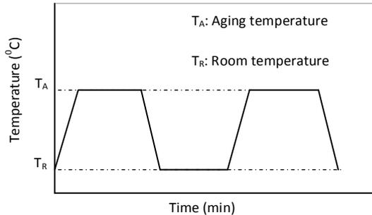
**Figure 6: time consuming discontinuous age hardening profile**
