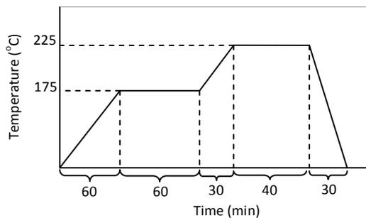
**Figure 3: Developed two step age hardening treatment with optimized parameters**
