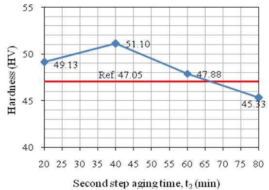
**Figure 4: Hardness Vs Second step aging time,  $t_2$**
