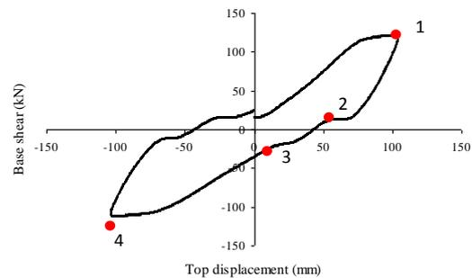
Figure 2: Base shear-top displacement hysteretic response
