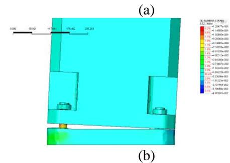
**Figure 4: (a) Deformation of each interface elements in reference to point 2 (b) Enlarged view of deformed shape in reference to point 2**
