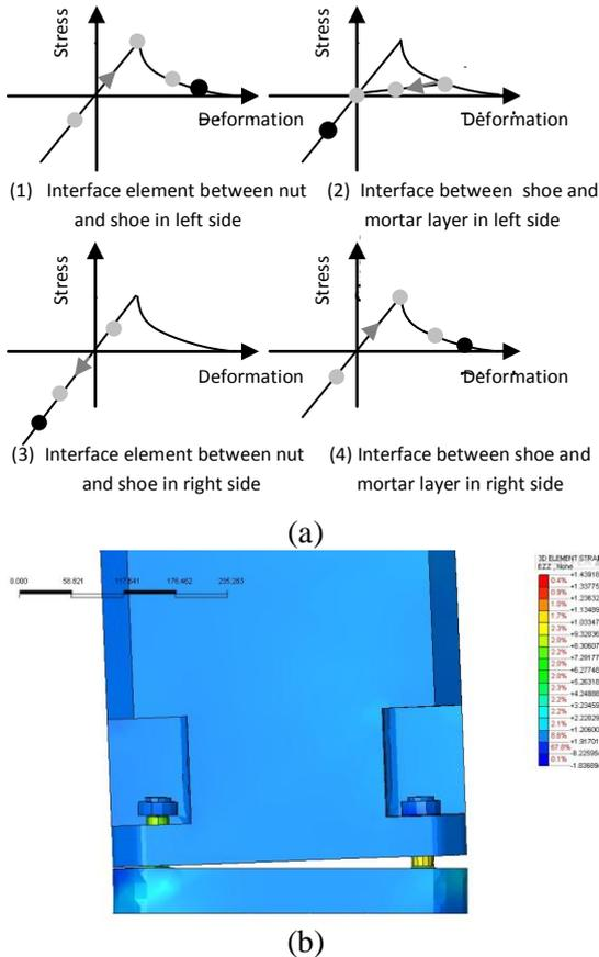
**Figure 6. (a) Deformation of each interface elements in reference to point 4 (b) Enlarged view of deformed shape in reference to point 4**
