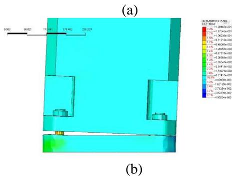
**Figure 3: (a) Deformation of each interface elements in reference to point 1 (b) Enlarged view of deformed shape in reference to point 1**
