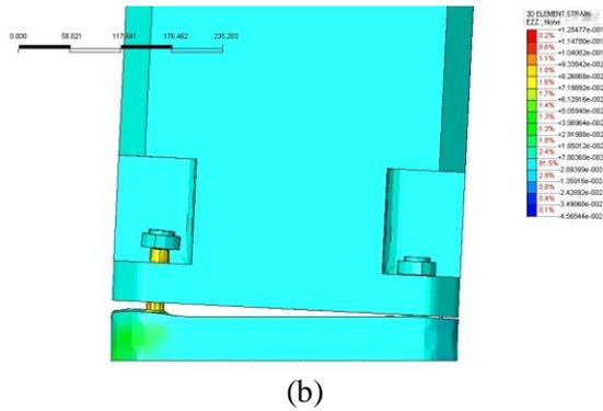
**Figure 5: (a) Deformation of each interface elements in reference to point 3 (b) Enlarged view of deformed shape in reference to point 3**
